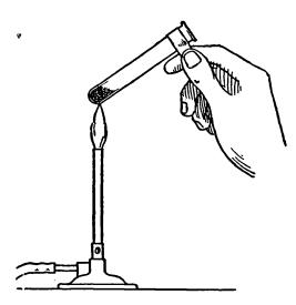
Fig. 5. The decomposition of mercuric oxide into mercury and oxygen by heat
